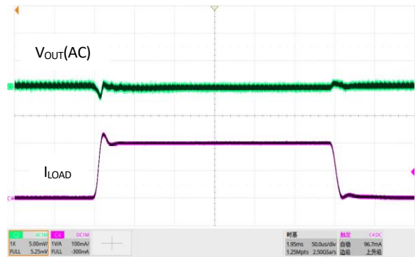
图 22. 负载瞬态响应, V_{IN}=4.3V , V_{OUT}=3.6V , I_{OUT}=5mA to 200mA
