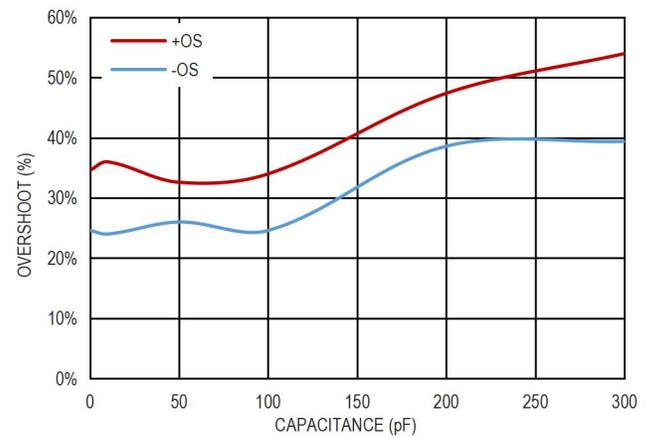
图 22. Small Signal Overshoot vs. Load Capacitance,  $V_S = \pm 2.5V$
