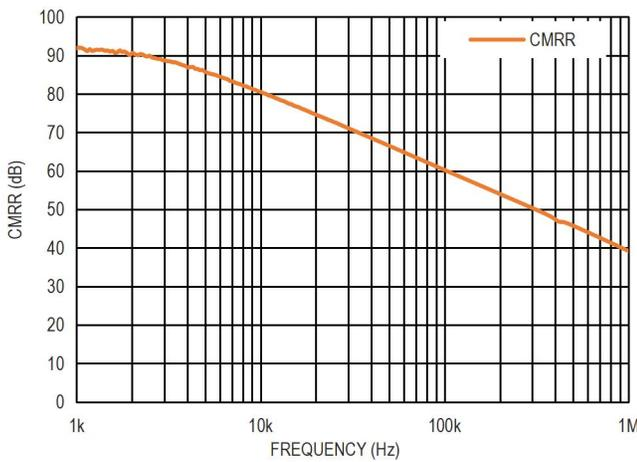
图 15. CMRR vs. Frequency,  $V_{IN}=28mV$ ,  $R_L=1M\Omega$ ,  $C_L=47pF$
