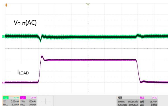
图 22. 负载瞬态响应, V_{IN}=4.3V , V_{OUT}=3.6V , I_{OUT}=5mA to 300mA
