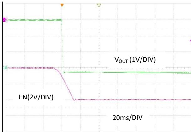
图 15. 软启动,  $V_{IN} = -4.3V$ ,  $V_{OUT} = -3.3V$ ,  $I_O = -500mA$
