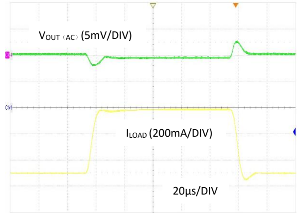
图 16. 负载瞬态响应, V_{IN} = -4.3V , V_{OUT} = -3.3V , I_{OUT} = 10mA to 500mA
